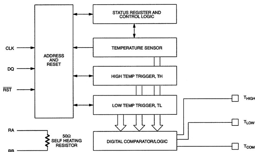
**TEMPERATURE MEASURING CIRCUITRY** Figure 2
