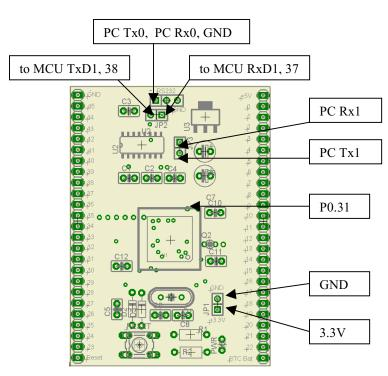
Note: The 3-Pin header connects to the MT PC serial download cable. JP2 connects to the second RS232 channel of MAX3232 IC and **not yet** wired to the ARMBoard's second RS232 channel (I/O Pin 37 & 38). JP3 connects to the second serial port of PC. Of course, all the Ground wires of all the devices MUST be connected together to act as the voltage reference point.
