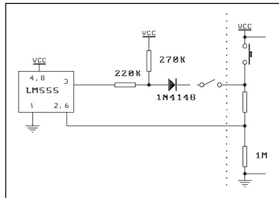
Add-on circuit to try. Components not supplied. Try to predict what will happen before you connect it. Just uses 220K & 270K resistor, LM555 and a 1N4148 diode.
