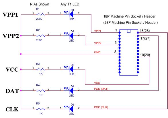
This tester, costing less than \$5USD, can test any socketed DIY PIC Programmer.
