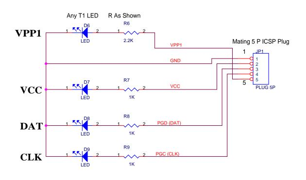
This tester, costing less than \$3USD, can test the DIY K182 PIC Programmer.
