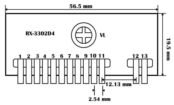
PIN 1 : GND PIN 2 : Digital Output
