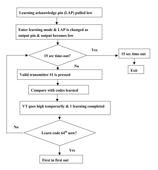
If 15 seconds of period is not long enough for learning all the transmitters, then the 2nd or the 3rd cycle of learning can be done until all the transmitters (up to 15 or 31 or 63 or 127 or 225 depending on which model of RX-3302D) is learned.
